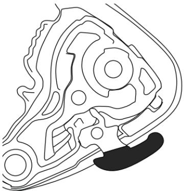
Note: When the lever is positioned at 3 o'clock, the shield is closed, but it is also unlocked.
